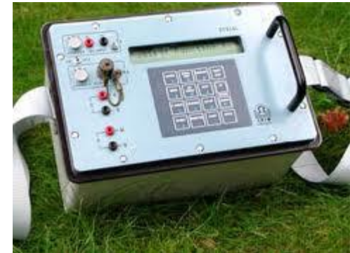
Electrical Sounding device 28
